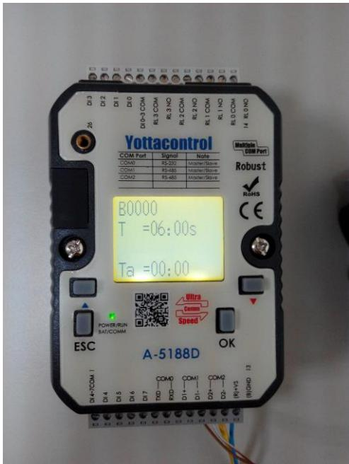
4. Current B0000 block is a timer and parameter is 6 Sec. Then press OK more than 3 Sec to adjust the timer.
