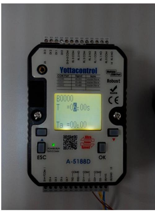
5. When finished the parameter adjust, press OK more than 3 Sec to save it.
